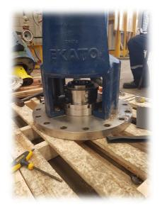
Step 2: Run the shaft through the seal and head out to the field
